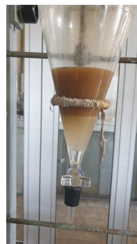
Fig. 5. Broken three - layer multicomponent liquid system.
