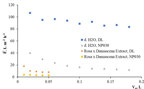
Fig. 2. Permeate flux in LMH ( $L m^{-2} h^{-1}$ ) versus cumulative permeate volumes for DL and NP030 nanomembranes during conditioning with distilled water and batch filtration of *R. damascena* extract at 10 bar transmembrane pressure.
