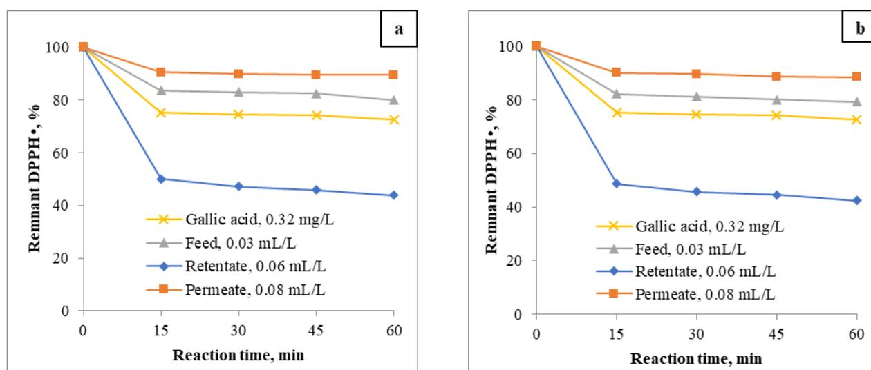
Fig. 3. Representative kinetics of radical scavenging reaction of gallic acid, *R. damascena* extract, and its nanofiltration fractions obtained with NP030 (a) and DL (b) membranes at indicated concentrations in the reaction mixture.
