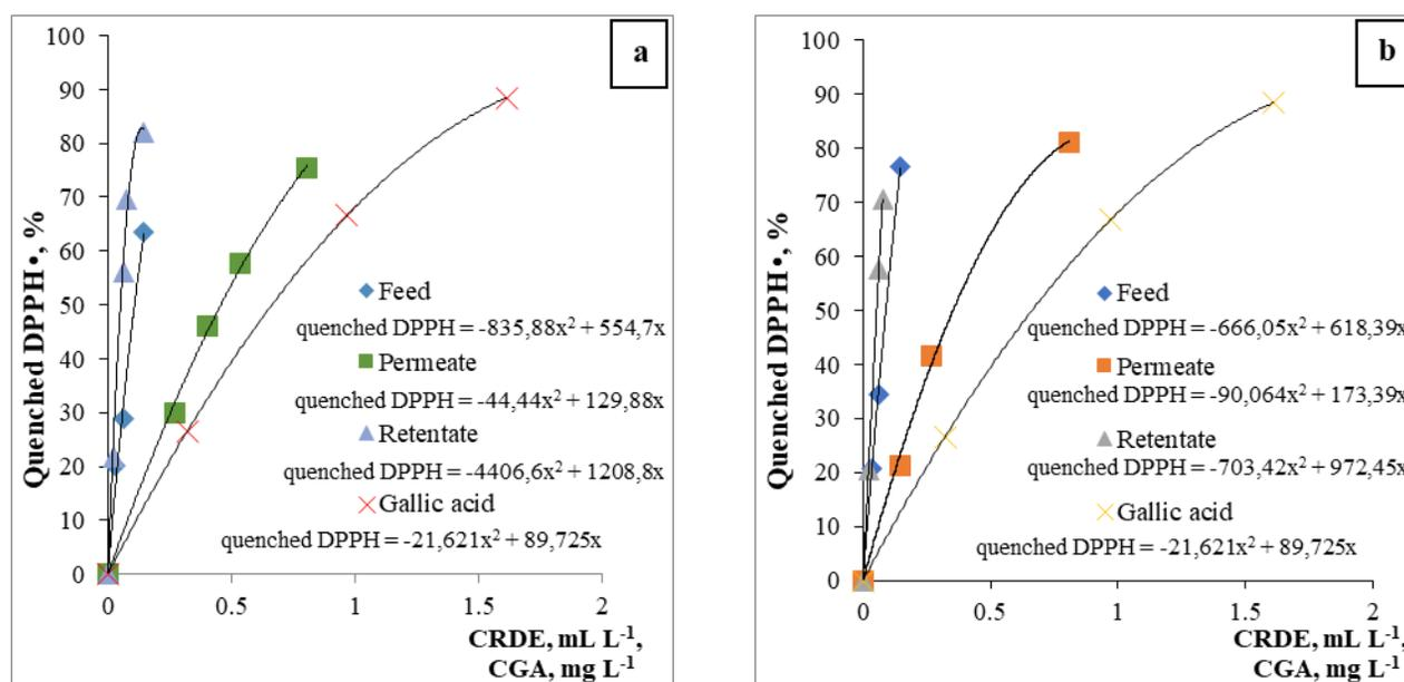
Fig. 4. Experimental data and curve fitting for DPPH• quenching in 60 min by *R. damascena* extract (RDE), its fractions filtrated by NP030 (a) and DL (b) nanomembranes and Gallic acid solution (GA) versus concentration of antioxidant in the samples.
