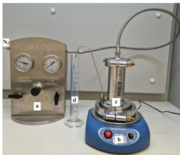
Fig. 1. Laboratory set-up for batch nanofiltration: a - pressure control unit; b - electromagnetic stirrer; c - nanofiltration cell (METcell); d - permeate vessel.
