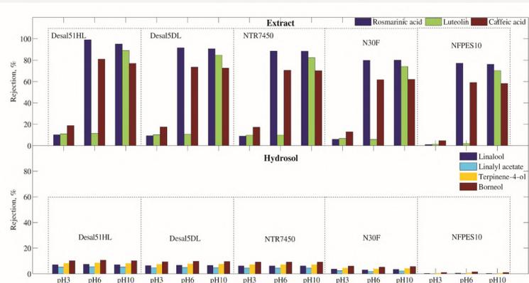
**Fig. 3.** Nanomembrane selectivity against key components of extracts and hydrosols from steam distillation of *Clove*
