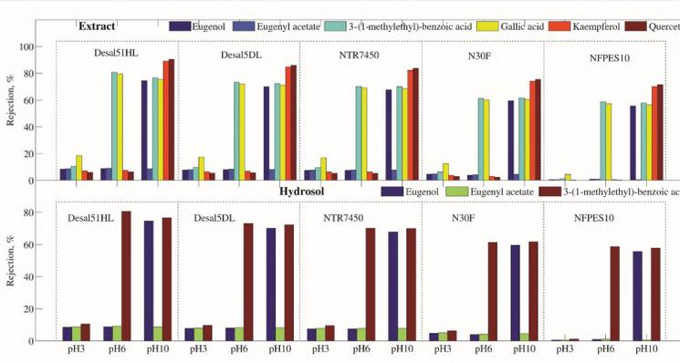
**Fig. 4.** Nanomembrane selectivity against key components of extracts and hydrosols from steam distillation of *Lemon balm*
